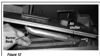
**Step 14.** Before you secure the burner with screws, double check that the orifice is positioned into the burner neck by feeling around the back of the burner (see *Figure 13*). Then, lower the burner so it sits flush on the burner supports and replace the 2 screws removed in step 6 (see *Figure 13*).
